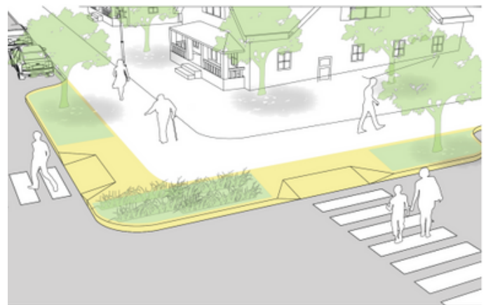
Figure 2: Example curb bulb-outs at intersections from the National Association of City Transportation Officials (NACTO).
